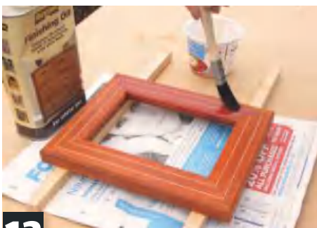
13 Brush on finishing oil and wipe off excess after a few minutes. Alternatively, simply apply a clear wax polish and buff
